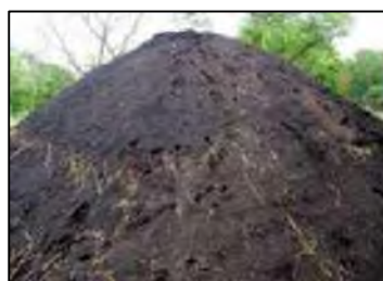
Figure1: Charcoal being produced by traditional earth mound kiln method
