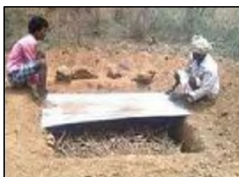
Figure2: Biochar being produced by pit kiln method
